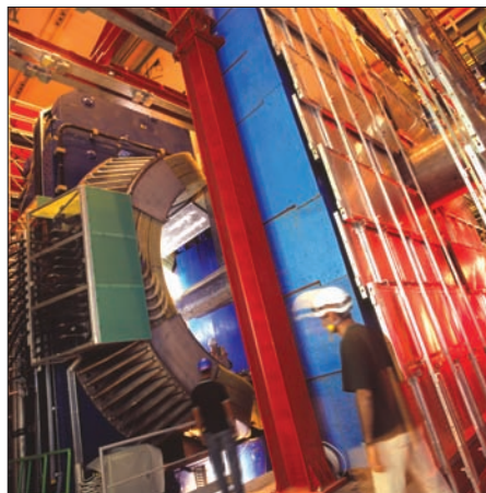
An ALICE trigger chamber is moved into position in front of the muon wall, with the dipole magnet in the background.
