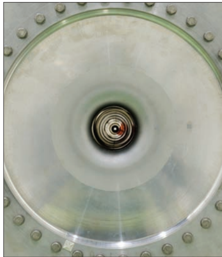
A view along the magnetic horn, prior to installation in the CNGS target chamber.
