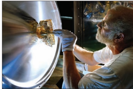
A technician carefully inserts the wakefield suppressor into LHCb's beryllium beampipe.
